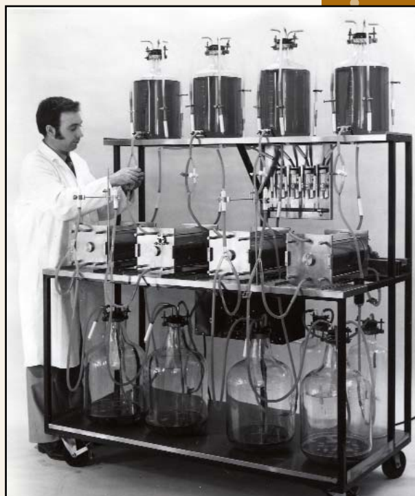
The Multi-Surface Cell Propagator, or MSCP, was based on an apparatus in which monkey kidney cells were grown on narrowly spaced glass discs mounted on a steel shaft that turned inside a glass cylinder. To maximize poliovirus production, several MSCP units were utilized together on specially designed portable carts.
