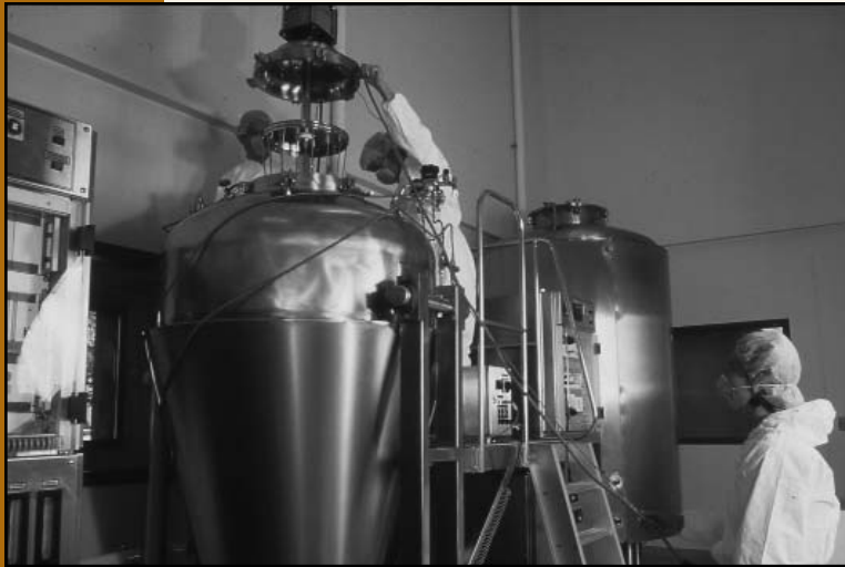
Since the early 1990s, Connaught's eIPV has been produced using poliovirus cultivated in microcarrier MRC-5 human diploid cell cultures inside specially designed, computer-controlled, 1,000 litre fermentor tanks. Source: sanofi pasteur limited
