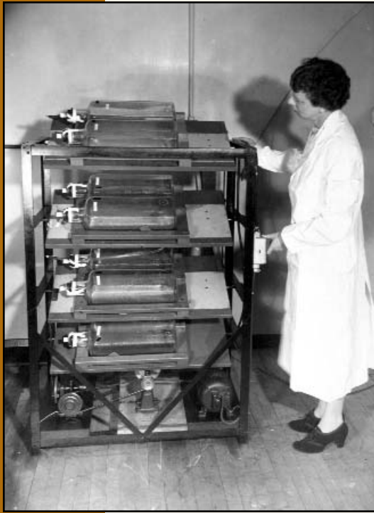
Dr. Leone N. Farrell applied her long experience with vaccine production at Connaught to the problem of large-scale cultivation of poliovirus fluids in monkey kidney cells and Medium 199 through the gentle rocking of large bottles in a custom-designed machine. Dr. Farrell is shown here next to the prototype rocking machine. Source: sanofi pasteur limited
