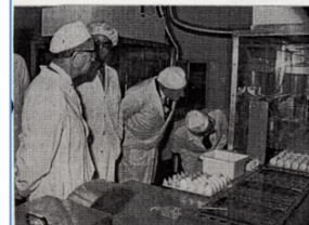
Dr. Jonas Salk and Dr. R.J. Wilson peer closely at the egg-inoculation machine in the influenza plant. This machine inoculates 36 eggs at one time.
